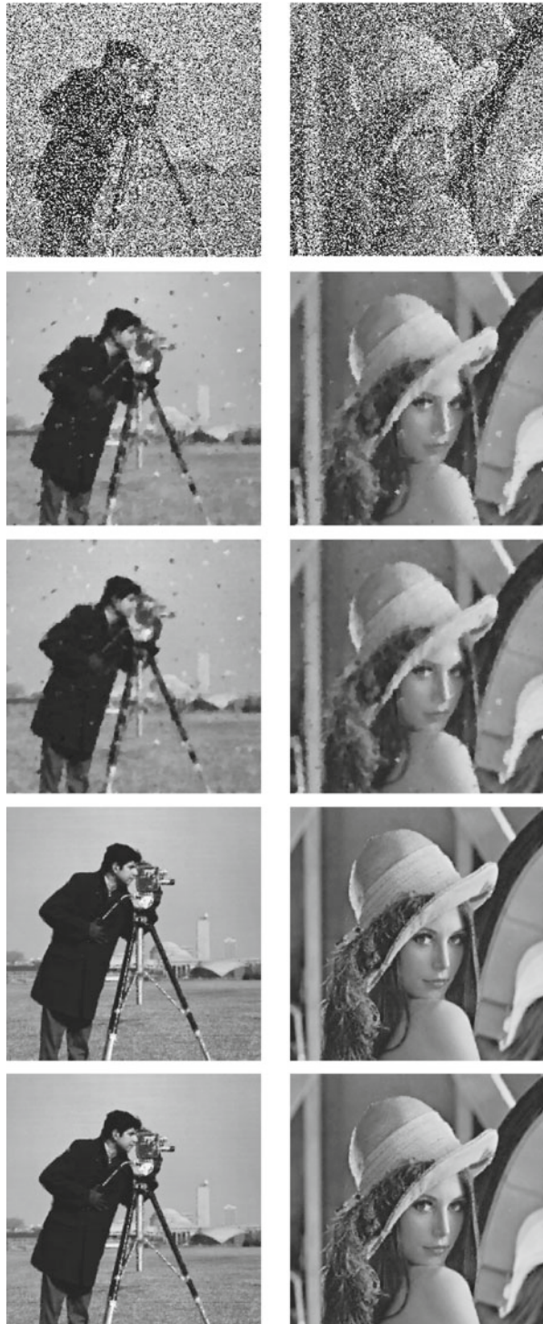
Fig. 4 Results of Algorithm 1 (Row 2), Algorithm 2 (Row 3), Algorithm 4 (Row 4) and Algorithm 4 (Row 5) when restoring noisy images (Row 1) are corrupted by salt-pepper noise with the noise level r = 50\% for the images of “Cameraman” and “Lena”
