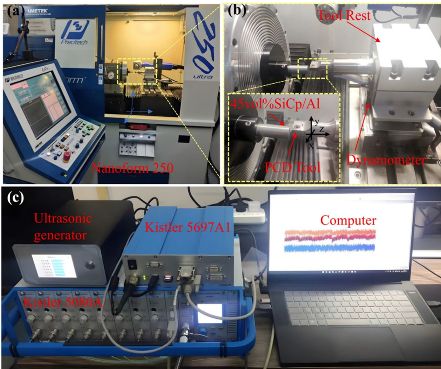
Fig. 6 Experimental setup for cutting SiCp/Al composites by UEVC: a Ultra-precision machine tool; b UEVC schematic; c force measurement system
