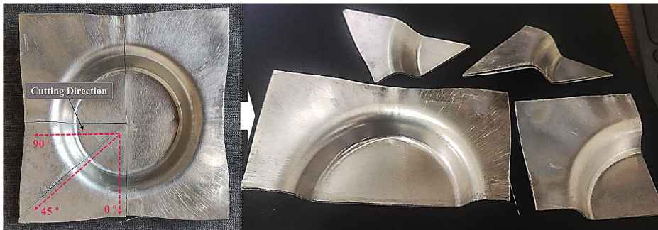
Fig. 9 FML cup cutting direction for wall thickness measurements
