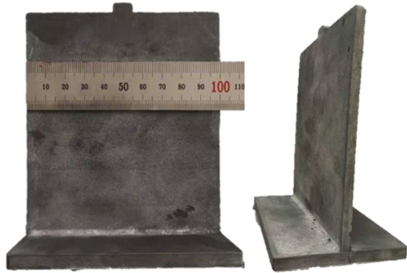
Fig. 17 T-shaped CF/Al composite part
