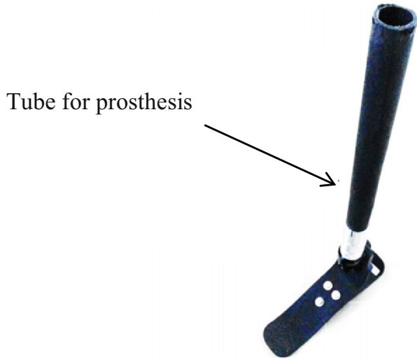
Fig. 1 Tube manufactured in epoxy/carbon composite material for transtibial prosthesis (Taken from [7])
