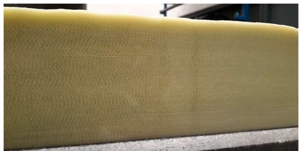
Fig. 9 A cut section of the thick composite laminate that has been examined in this study
