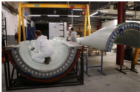
Fig. 1 Full-scale tidal turbine blade during manufacture that is detailed in this study
