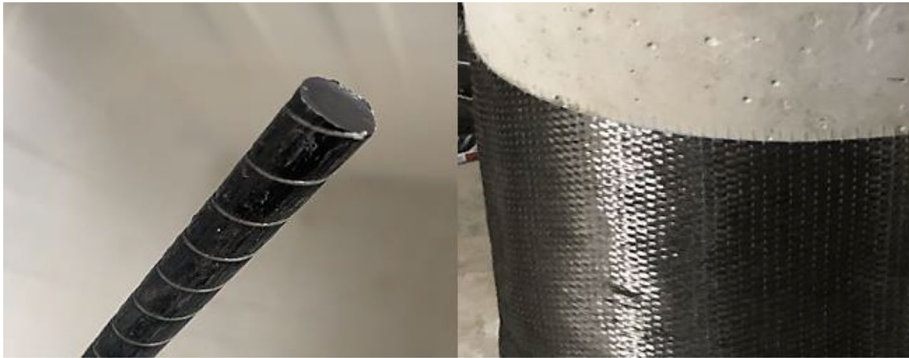
Fig. 1 The CFRP bar and CFRP sheet for testing
