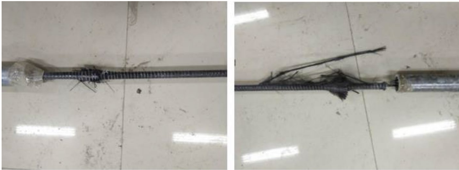
Fig. 5 The failure mode of CFRP bars
