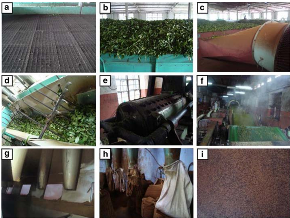
Fig. 3 Step-by-step extraction process of TLF. a Wire mesh; b Fresh tea leaves are laid out on the wire mesh; c Hot air forced through the bottom of fresh leaves; d Tea leaves flow to the rotor vane; e CTC machine (crushing, tearing, and curling); f Completely crushed tea leaves move to the conveyor; g Particulate tea leaves flow to the fluid bed drier; h Using exhaust fan, fine particles of tea leaves are carried away from the drier; i Extracted bio-degradable WTLF
