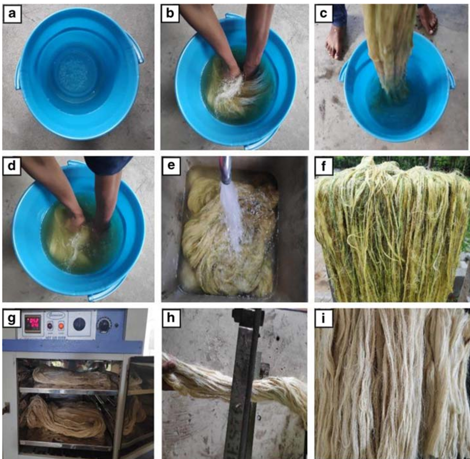
Fig. 4 Schematic representation of the alkali treatment process. a 5% alkali solution; b Fibers dipped into alkali solution for 3 h; c Fibers are rinsed with the water; d Fibers washed with diluted HCL; e Fibers are cleaned with running water several times; f Fibers are dried with sunlight; g Fibers are placed in a hot oven with temperature range of 70 °C; h Fibers are cut using hand shearing machine; i Final length of the fiber is 300 mm
