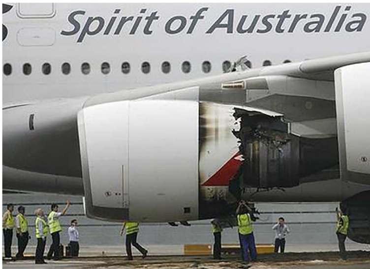
Fig. 2 An engine blows up on a new Airbus A380 on Qantas Airline flight 4 November 2010. A turbine disc in the Rolls-Royce Trent 900 engine disintegrated resulting in damage to the nacelle, wing, fuel system, landing gear, flight controls, and undetected fire in an inner wing fuel tank. Failure was caused by fracture of a stub oil pipe
