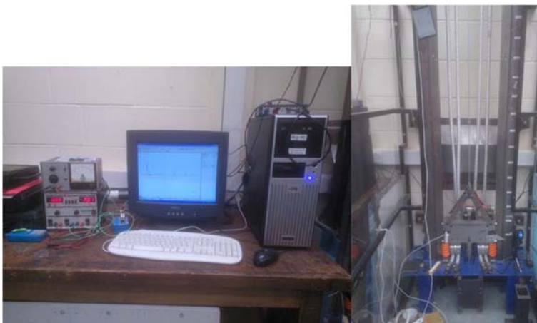
Fig. 4 Drop tower impact machine used during the experimental campaign
