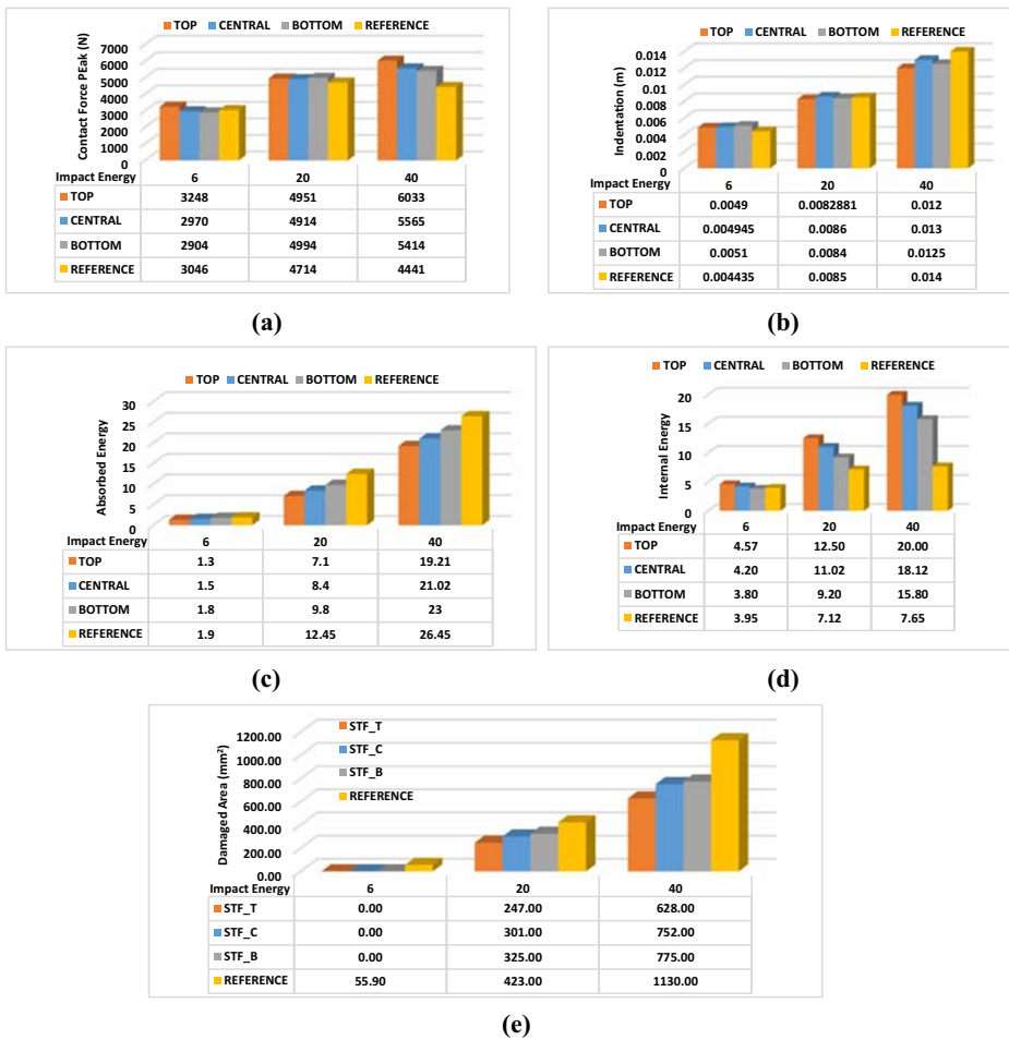
Fig. 10 Impact results from experimental and numerical tests: (a) Maximum contact force, (b) Maximum displacement, (c) absorbed energy, (d) internal energy and (e) Damaged area extension
