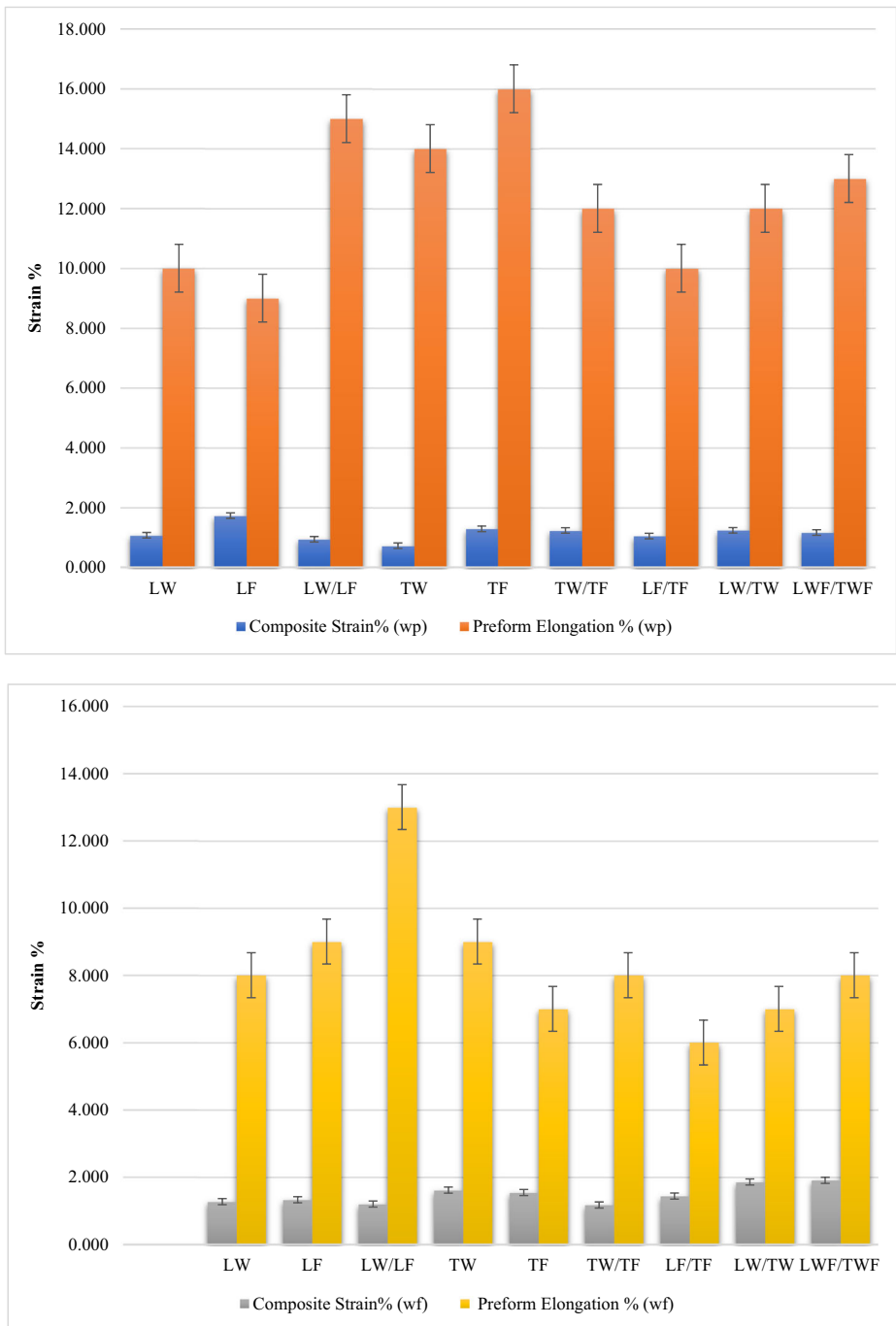
Fig. 5 Elongation % (at break) of the preform and strain % (at break) of composites in warp and weft directions
