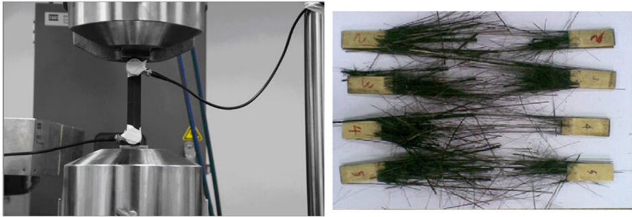
Fig. 9 The tensile experiments of unidirectional carbon fiber/epoxy composite specimens
