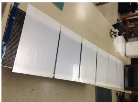
(a) Nanocomposite film placed on the carbon fabric
