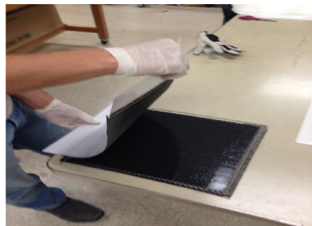
(b) Stacks of carbon Fabric with Nanocomposite film as interleave
