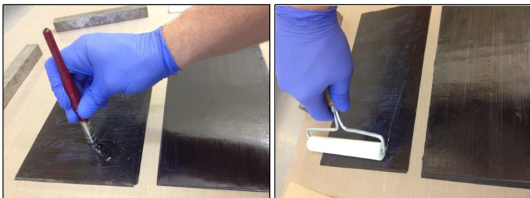
Fig. 7 manufacturing procedure of STF/CFRP composite samples
