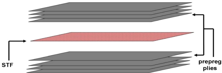
Fig. 6 Schematics of STF/CFRP composite preparation
