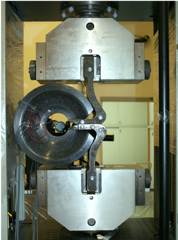
Fig. 6 Test machine setup; Zwick Z250 Universal Testing System, load transfer elements and the scaled CFRP rotor
