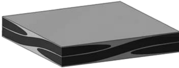
Fig. 1 Representative volume element (RVE) of woven composite
