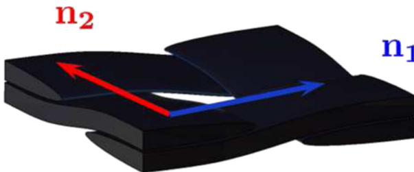
Fig. 2 Woven fibers and definition of fiber directions n_1 and n_2
