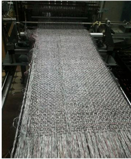
Fig. 2 Weaving machine and 3D warp interlock preform with E-glass/PP commingled yarns
