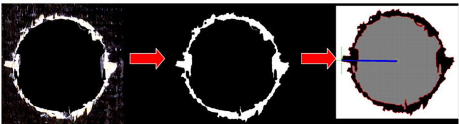
Fig. 8 Digital image processing of delamination
