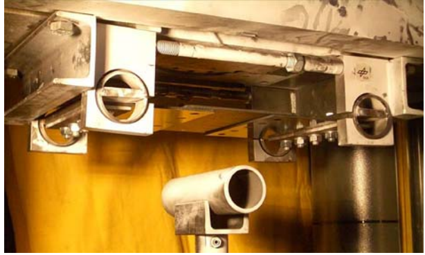
Fig. 16 High-rate line load test fixture
