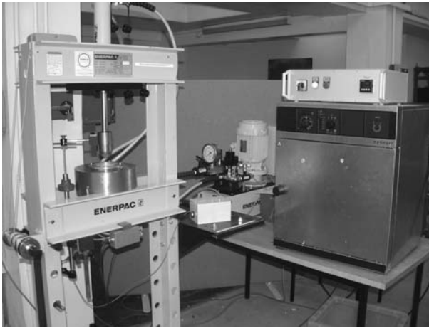
Fig. 3 Photograph of the non-isothermal hydraulic stamping press used to produce hemispherical all-PP domes. The preheating oven is shown on the right hand side of the photograph, while the stamping press is shown on the left. Figure 4 shows a more detailed photograph of the matched metal mould used to form the all-PP domes
