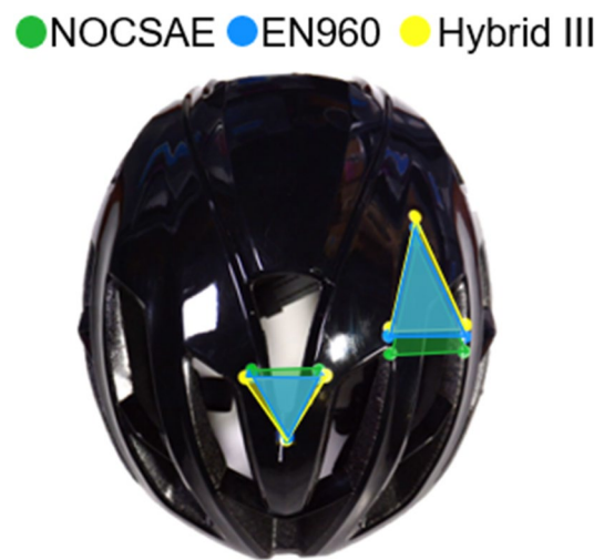
Fig. 2 Comparison of impact locations for each headform (NOCSAE (green), EN960 (blue), Hybrid III (yellow)) and two primary orientations (y-axis and x-axis rotation, SAE J211 standard coordinate system). A custom 3-laser system was mounted onto the anvil to allow impact locations to be marked as each helmeted headform was positioned accordingly
