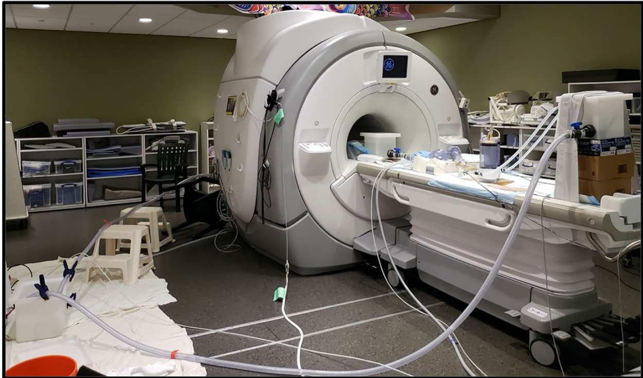
Fig. 1 Experimental flow loop setup on the MRI magnet table in the Richard M. Lucas Center for Imaging at Stanford University
