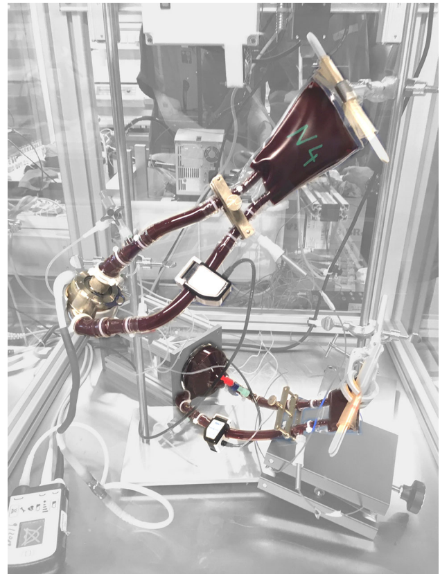
FIGURE 1. Set-up of Mini test loops with HM3 (top) and BPX-80 (bottom).
