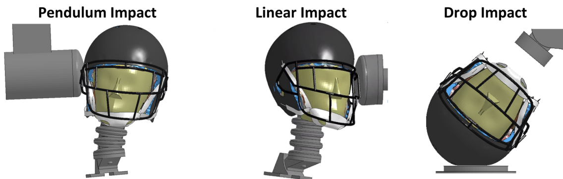
FIGURE 3. Visual overview of the three impact conditions used for helmet validation. HIII head form is shown.
