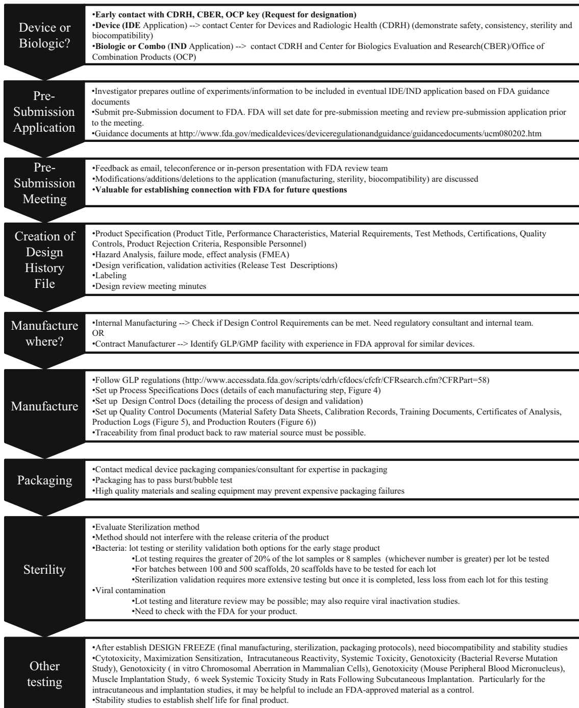
FIGURE 2. Flow chart listing steps to successfully get through an IDE application for a medical device at the FDA.
