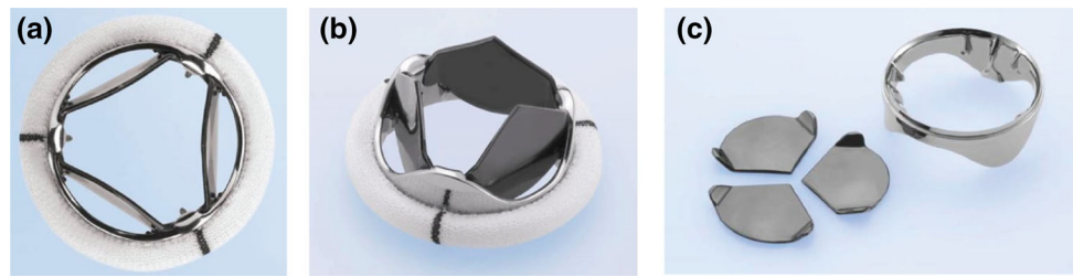
FIGURE 2. A trileaflet mechanical heart valve provides flow characteristics that more closely mimic native aortic valves. The valve contains a pivot mechanism that allows airfoil-like leaflets to close before flow reverses, a phenomenon that also occurs in the body. (a) Valve from above in fully open position. (b) Elevated isometric view of the valve in a fully open position. (c) Disassembled valve with three pyrolytic carbon leaflets and ring. Images are courtesy of Ulrich Steinseifer, Helmholtz Institute, Aachen, Germany.
