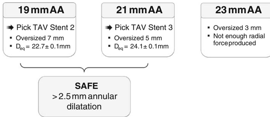
**FIGURE 7.** Transcatheter valve stent–tissue pairings. Oversize measure and corresponding equilibrium diameter position ( $D_{eq}$ ) for TAV stents offering an expansion force that meets the minimal required annulus dilatation to counter migration in non-calcified aortic tissue.
