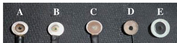
FIGURE 1. Five common types of Ag/AgCl bio-electrodes tested in the experiment.
