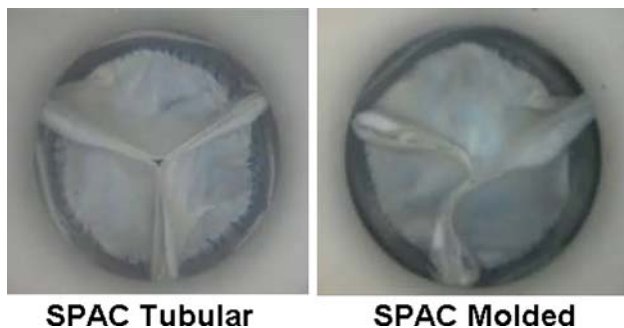
FIGURE 4. Images of the SPAC tubular valve and the SPAC molded valve in the fully closed position captured from the in vitro video results.
