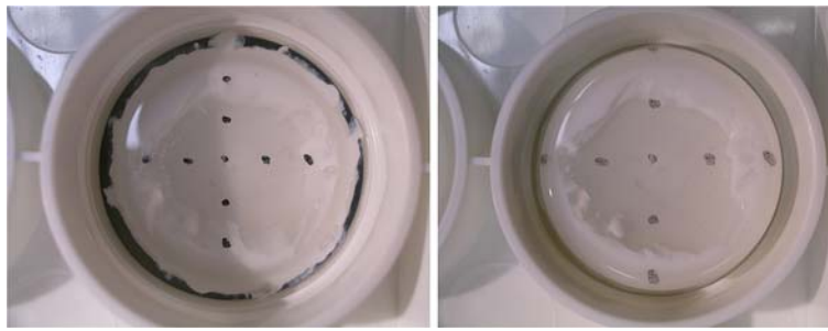
FIGURE 2. One example of a single well in the unstretched position (left) and 2.54 cm indenter depth corresponding to approximately 100% \Delta SA (right).
