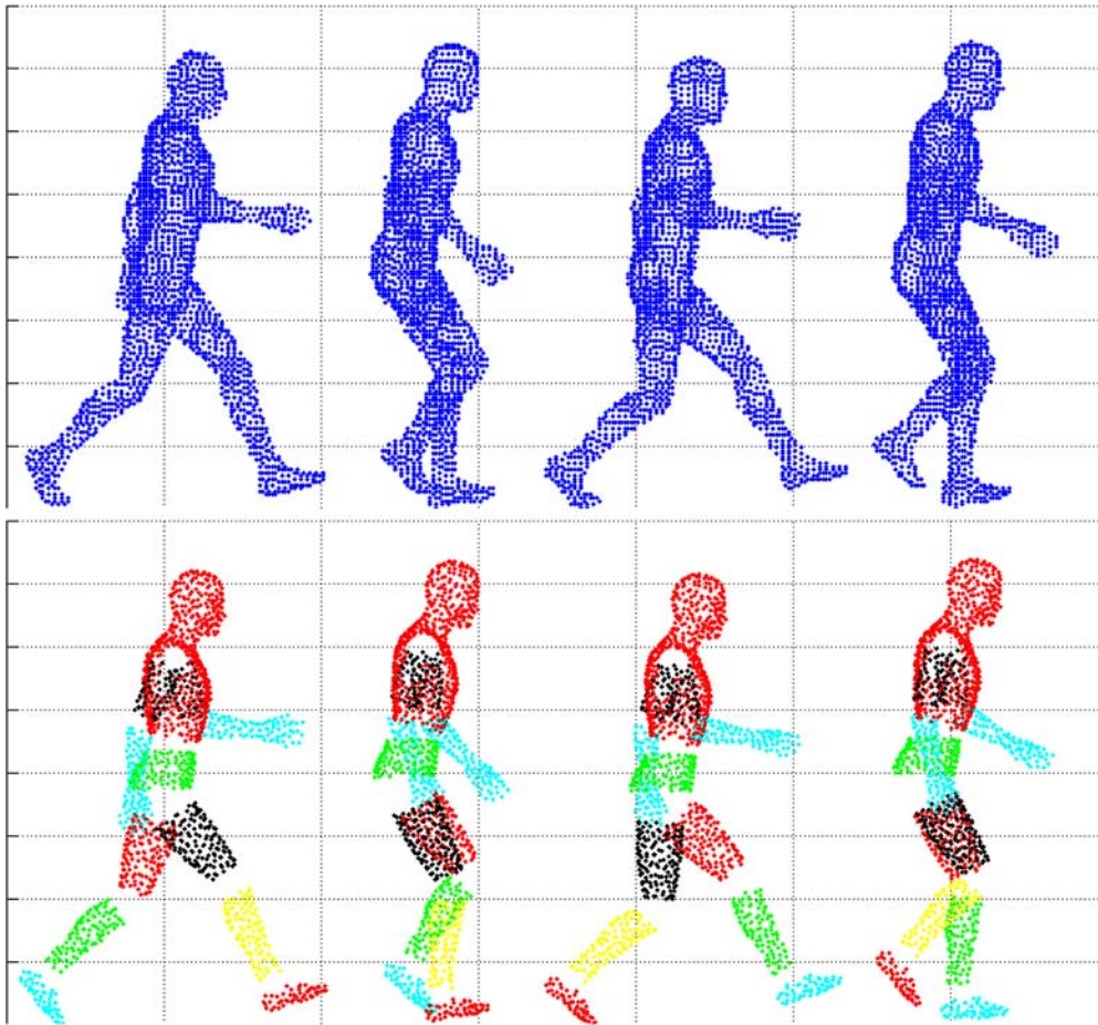
FIGURE 4. Results of the matching algorithm applied to the virtual environment sequence. Points visual hull (top, in blue) and matched model (bottom) for a gait cycle, in the sagittal plane.
