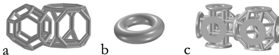
FIGURE 2. Illustration of the need for a common interface between building blocks. (a) Example of two polyhedra lacking a common interface. Notice that at the interface between the two polyhedra, no material interaction occurs. (b) A torus used for the common interface between building blocks. (c) Example of the matching between two dissimilar polyhedra containing a common interface of a split torus.
