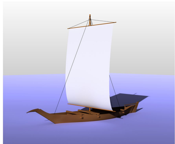
Fig. 25 3D digital model of Shungwaya at a draft of 0.91 m (Rhinoceros 3D® software)
