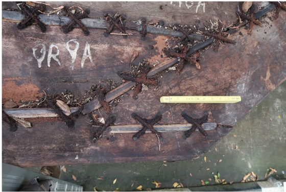
Fig. 16 Scarf between the keel and the stem
