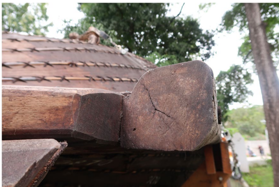
Fig. 14 Aft extremity of the keel, at the stern. Image not to scale
