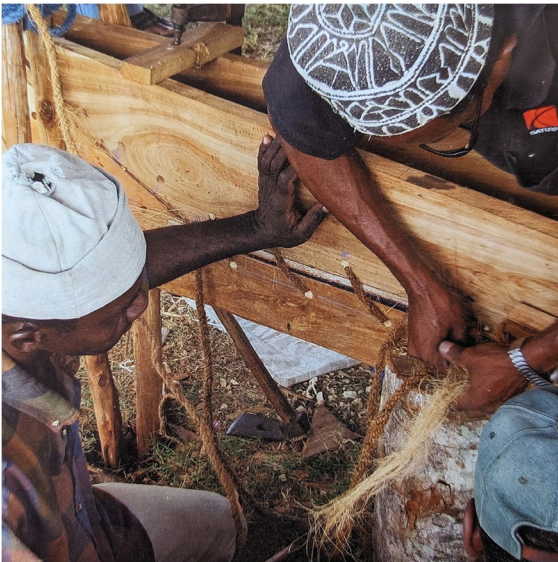
Fig. 9 Sewing the garboard to the keel with a coir rope. Modified after the House of Wonders and Zanzibar National Museum of History and Culture (2004)
