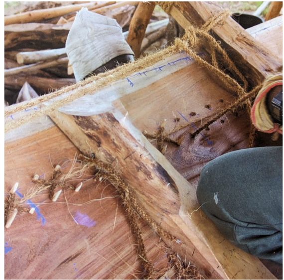
Fig. 10 Sewing the planks along the seams. Note the pre-drilled holes along the seams being plugged with pegs from the outside, and the frames being installed. Modified after the House of Wonders and Zanzibar National Museum of History and Culture (2004)
