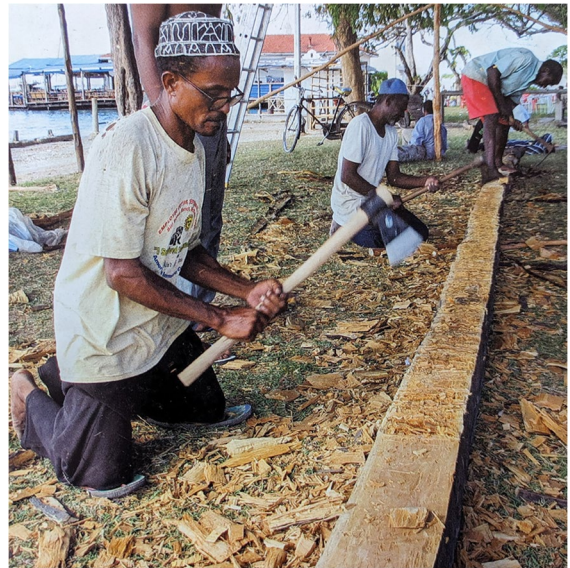
Fig. 6 Shaping of the keel with adzes. Modified after the House of Wonders and Zanzibar National Museum of History and Culture (2004)
