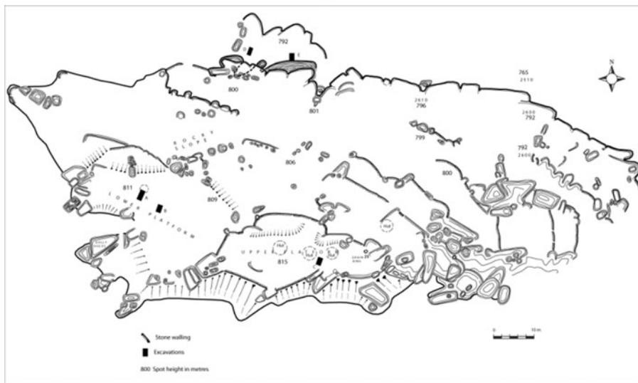
Fig. 2 Garlake's (1968) map of Mapela summit showing multiple platforms covering the entire hilltop. The platforms are built of poorly coursed dry-stone walls and contain solid dhaka structures. A preliminary house count identified at least 24 houses on the different platforms
