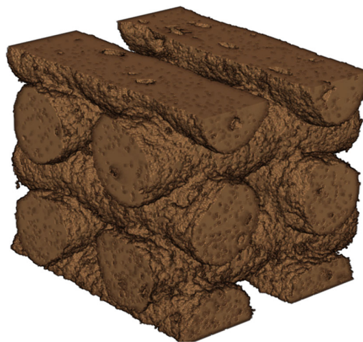
Fig. 3 3D geometric model based on \mu - CT scans of the printed scaffold
