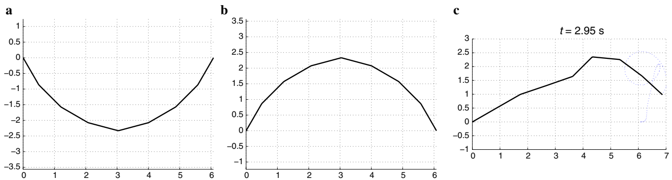
Fig. 8 Shape control of an 8-segment model: simulation for “reversing an arch”. a Initial shape, b disired shape, c final shape attained at t = 2.95 s
