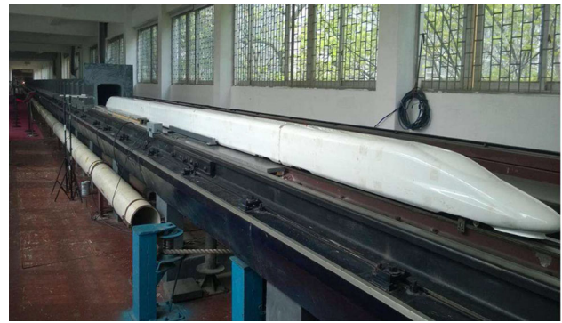
Fig. 19 Moving model test for train going through a tunnel
