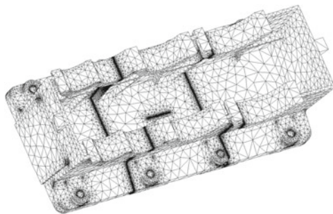
Fig. 9 A gear box meshed with elements of smaller size at specific locations
