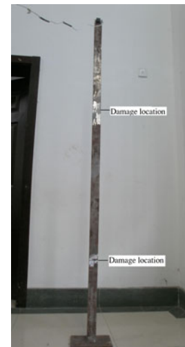
Fig. 8 The tested beam structure used in the experiment
