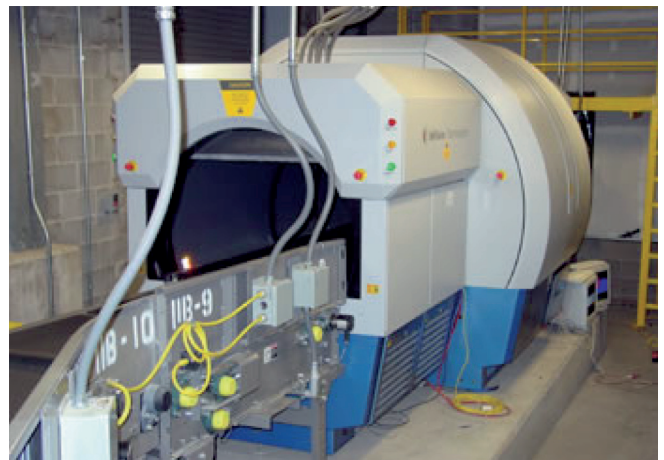
Fig. 11 Explosives Detection System (Turner Construction Company, USA), a CT scanner for detecting suspicious object in checked flight baggage ( http://www.turnerconstruction.com/aviation/content.asp?d=3247&p=3245 , with permission)
