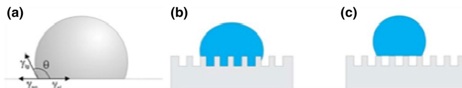
Fig. 2 a Surface tension of a water drop on a smooth surface; b Wenzel state: penetration of liquid droplet into surface irregularities; c Cassie–Baxter state: trapped air makes liquid drop suspend on the
