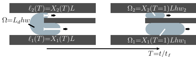
Fig. 4 Top-view schematic of a drop colliding with an obstacle defining the variables used in our model which describes the propagation of two-liquid interfaces in the two gaps
