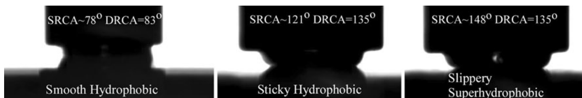
Fig. 5 Drop shape and contact line under equilibrium state with flow/extraction set and the water drop sitting on various surfaces
