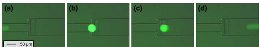
Fig. 12 A large fluorescent particle passing through the 50 µm valve with a flow rate of 40 µl min -1
