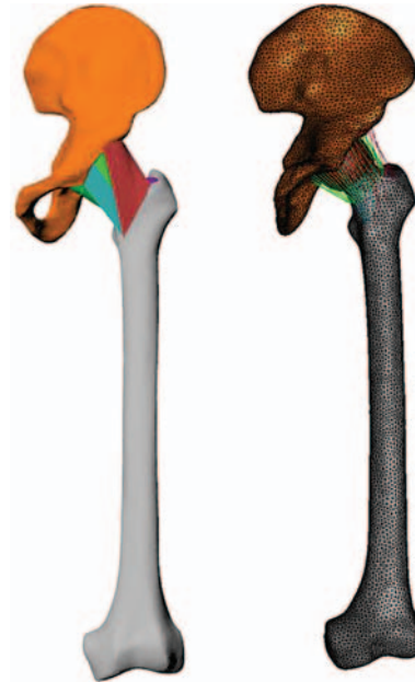
Fig. 2: Complete geometric model of the hip (left) and computational FEM model (right)
