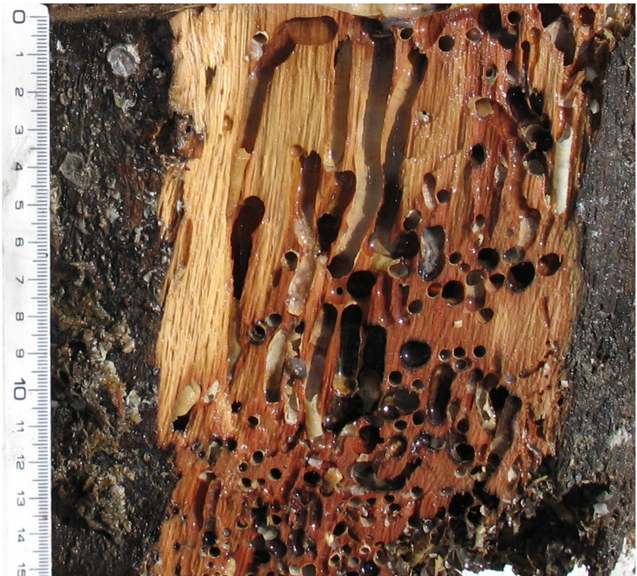
Fig. 2 Section of an Oak pole subjected to shipworm attack. The tunnels follow the grain of the wood upwards and are plastered with a calcareous coating secreted by the molluscs
