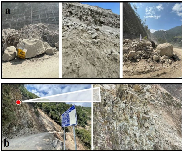
Fig. 9 Landslides with different lithologies in the study area a loose gravel layer, b granite
