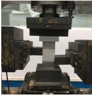
Fig. 2 Rock physical and mechanical parameters test
