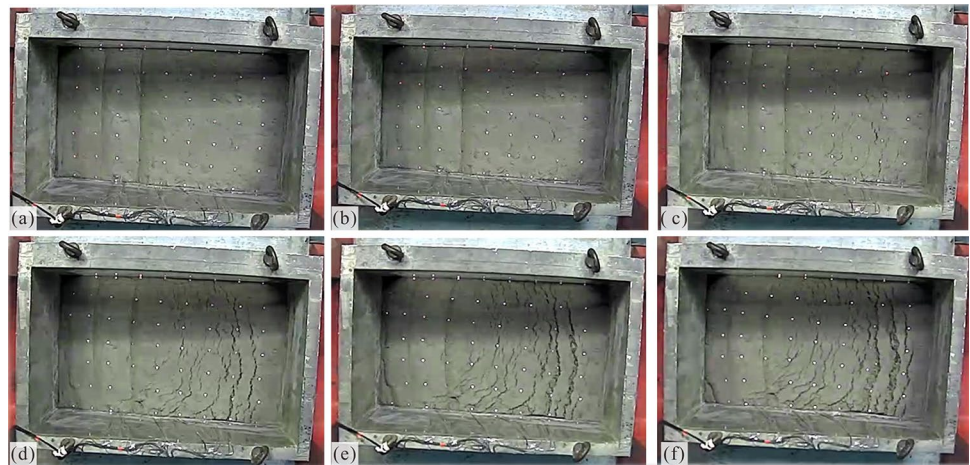
Fig. 7 The development process of cracks on the slope surface of the LST-2 test model when the water content is 15%. a The time is 7 min, and the acceleration is 30 g; b the time is 9 min, and the acceleration is 40 g; c the time is 10 min, and the acceleration is 50 g; d the time is 12 min, and the acceleration is 60 g; e the time is 14 min, and the acceleration is 80 g; f the time is 19 min, and the acceleration is 100 g
