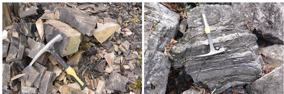
Fig. 7 Failure mechanism of the sources I and II. The sliding directions of the sources were the inclination of the unconformity contact interface and the apparent dip of the limestone strata respectively. The source I as a “key resistance block” determined the overall stability of the WRA
